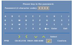
CHANGE PASSWORD—Key in the original password, then enter the new password and confirm the new password again.
