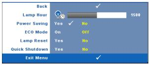
LAMP HOUR—Displays the operating hours since the last lamp timer reset.
